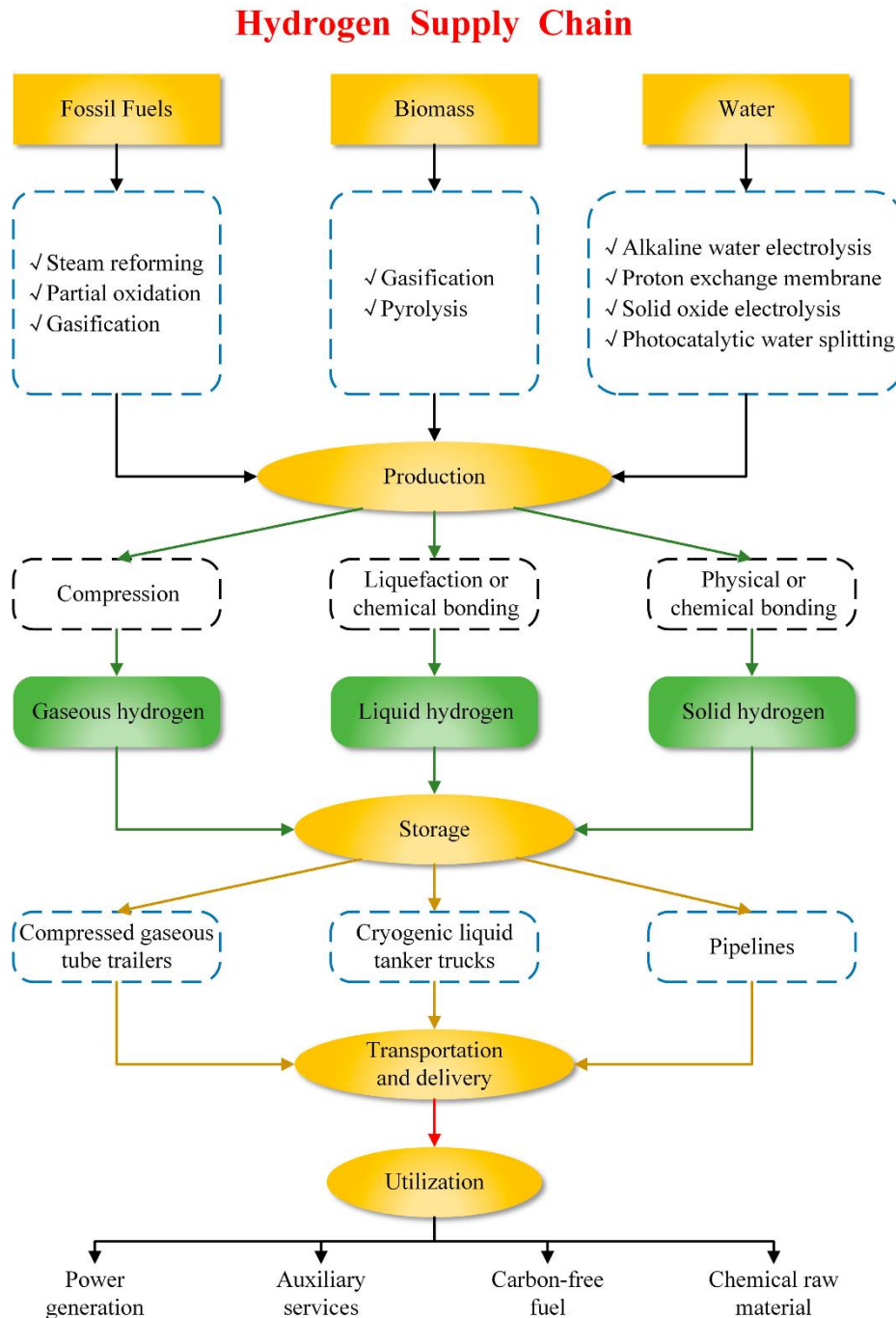
Figure 1: Key components of a hydrogen supply chain
